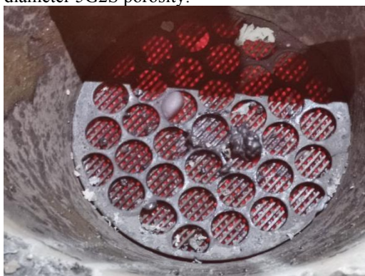
Fig. 5 shows a MetCon C filter after almost 3 tonnes of molten steel have been poured through it. The filter is a 200 mm tapered
