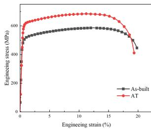
Fig. 2 Tensile engineering stress-strain curves of As-built and AT Fe-Ni-Co-V Invar specimens.
