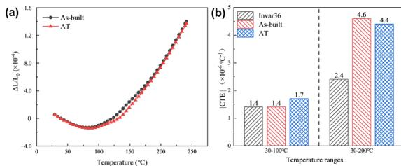
Fig. 3 (a) Thermal expansion curves of As-built and AT Fe-Ni-Co-V Invar; (b) absolute value in different temperature ranges of Invar36, As-built and AT Fe-Ni-Co-V Invar.
