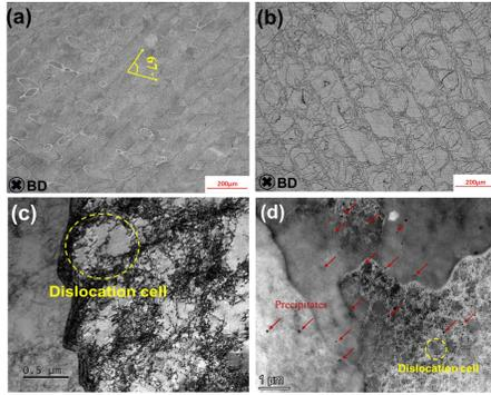
Fig. 1 OM micrographs of (a) As-built Fe-Ni-Co-V Invar; (b) AT Fe-Ni-Co-V Invar and TEM micrographs of (c) As-built Fe-Ni-Co-V Invar; (d) AT Fe-Ni-Co-V Invar.
