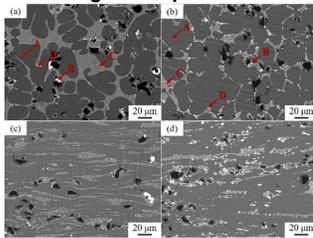
Fig.2 BSE micrographs of the 0Mg ((a)as-cast, (c)as-rolled) and 2Mg ((b)as-cast, (d)as-rolled) composites
