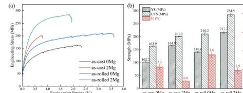
Figure 3 (a) Engineering stress-strain curves and (b) detailed mechanical properties.
