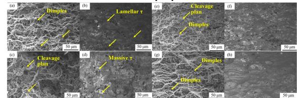
Figure 4 SE and BSE fractography of the as-cast 0Mg(a-b), 2Mg(c-d), as-rolled 0Mg(e-f), and 2Mg(g-h) composites.
