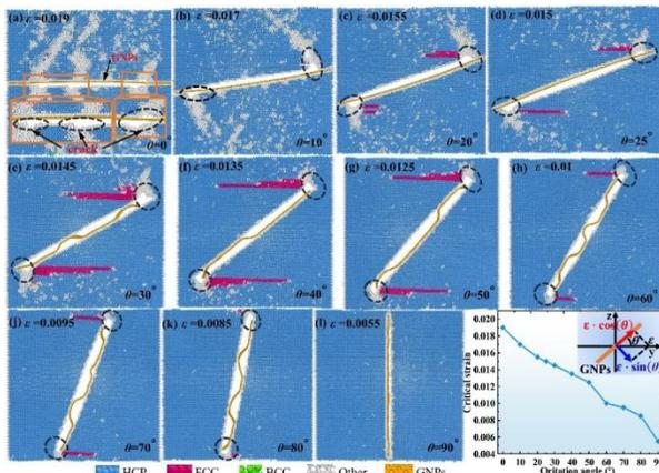
Fig.2 The evolution morphology of AZ91/GR composites with different orientation angles of GR under critical strain.
