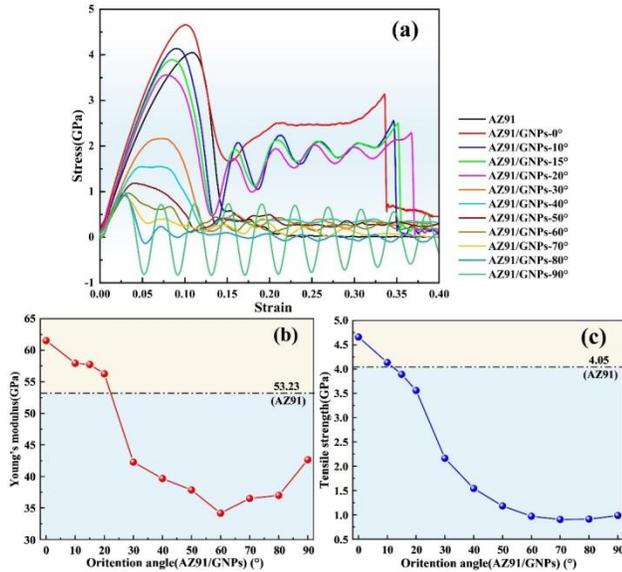
Fig.1 (a) The stress-strain curves of AZ91 alloy and AZ91/GR composites were measured at different orientation angles of GR; (b) The Young's modulus of the composite material depicted in the fig. (a); (c) The tensile strength of the composite material depicted in the fig. (a)
