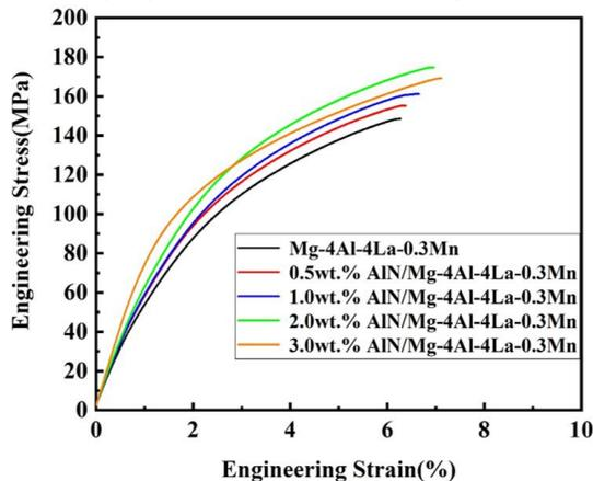
Figure 3. Room temperature tensile engineering stress-strain curves of AIN/AE44 composites.
