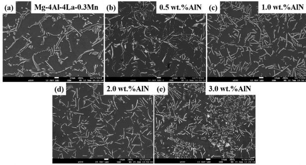
Figure 2. Microstructure images of AIN/AE44 composites with different AIN content
