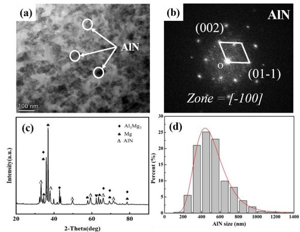
Figure 1. In-situ AlN/Mg master alloy: (a) TEM image, (b) SAED image, (c) XRD results; (d) size statistics diagram of AlN particles.
