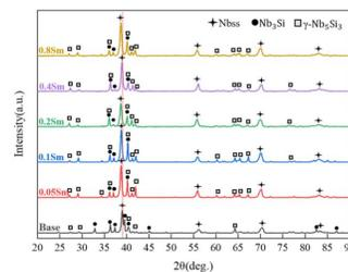
Figure 1 XRD patterns of base-xSm (x = 0, 0.05, 0.1, 0.2, 0.4, and 0.8) alloys
