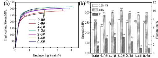
Figure 3 (a) Engineering stress-strain curves and (b) detailed mechanical properties of T6-samples.
