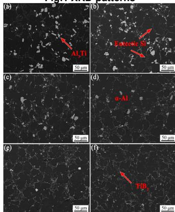
Fig.2 SEM (BSE) micrographs of the composites: (a) 5-0#; (b) 4-1#; (c) 3-2#; (d) 2-3#; (e) 1-4#; (f) 0-5#
