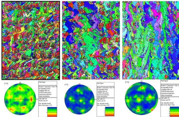
Fig. 2 EBSD maps of DED fabricated IN 718 samples with varied magnetic field intensities.
