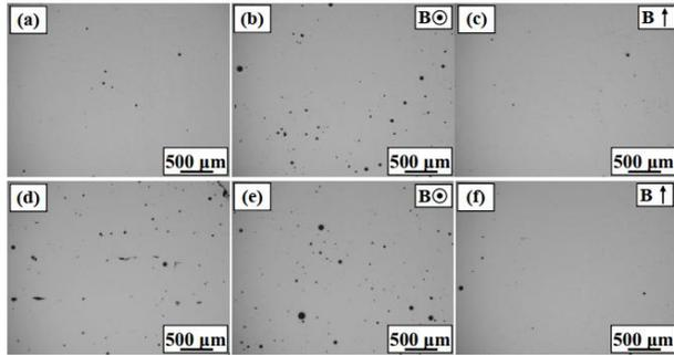
Fig. 1 Optical microscope of Inconel 718 alloys processed using different laser energy density and SMF intensities.
