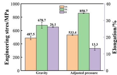
Fig. 4 Room temperature tensile properties of as-cast K4169 alloy under different casting processes
