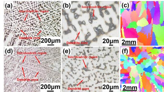
Fig. 3 Comparing the casting methods on the microstructure and grain morphology of as cast K4169 alloys: (a)-(c) Gravity investment casting; (d)-(f) Counter gravity adjusted pressure investment casting.
