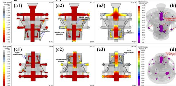
Fig. 2 Comparing the solid phase fraction distribution at different time points (a and c) and defect distribution (b and d) during traditional gravity casting (a-b) and counter gravity casting (c-d) by numerical simulation.
