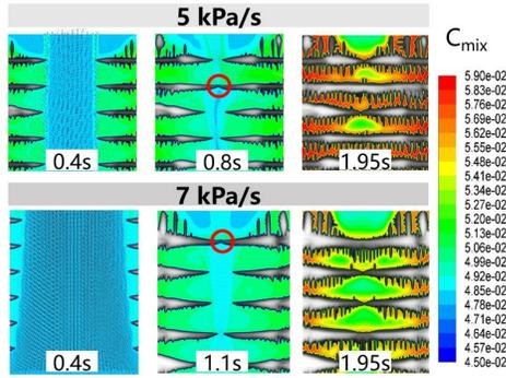
Fig. 1 Dendrite evolution in thin-wall structure with various pressure during counter-gravity casting.
