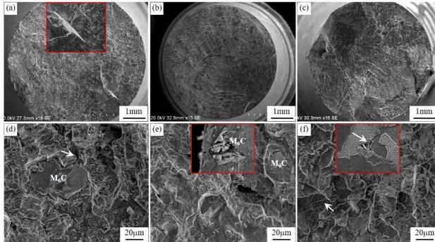
Fig. 2 SEM morphology of the alloy after high-cycle fatigue fracture at different temperature: (a)(d)800 °C, (b)(e)900 °C and (c)(f)1000 °C
