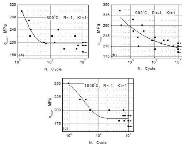
Fig. 1 High-cycle fatigue S-N curve of the alloy at different temperature: (a)800 °C, (b)900 °C and (c)1000 °C
