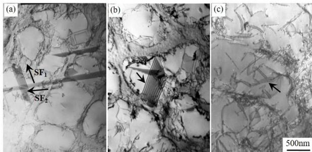
Fig. 3 TEM morphology of the alloy after high-cycle fatigue fracture at different temperature: (a)800 °C, (b)900 °C and (c)1000 °C
