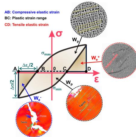
Figure 2. Schematic diagram of the calculation method of total strain energy as well as the relationship between the energy composition and typical deformed microstructures.
