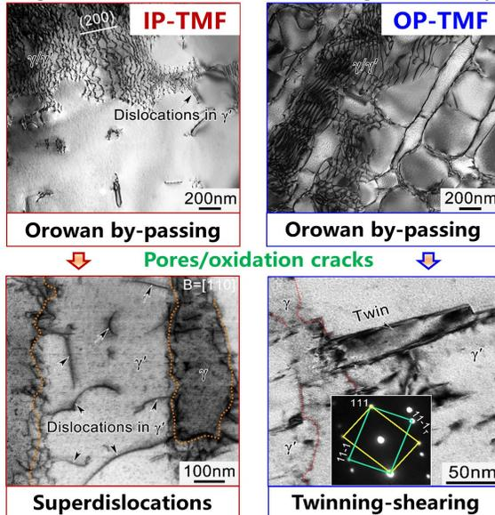
Figure 1. Evolution of dislocation configurations when pores or oxidation cracks were introduced during TMF.
