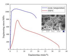
Figure. 2 Engineering stress-strain curve of alloy.
