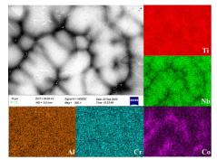
Figure 1. As cast microstructure and EDS analysis of alloys.
