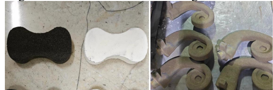
FIG.1 Core for tensile strength sample and core forming effect evaluation
