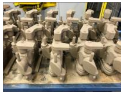
Figure 3: left: series of sand cores to be casted; right: smooth and sand-free casting surface.
