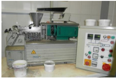
Fig. 2 Laboratory extruder for foundry powder coatings manufacturing
