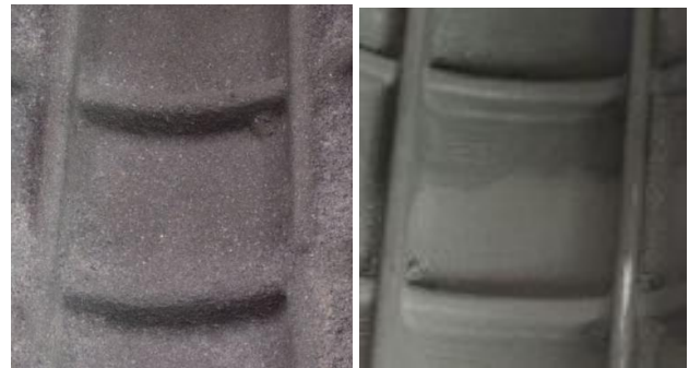
Figure 4 Casting result in variation of HD coating A and HA coating B
