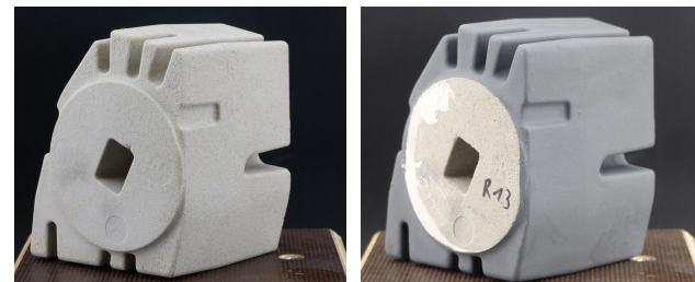
Figure 1 Core design – coated and uncoated for cast node
