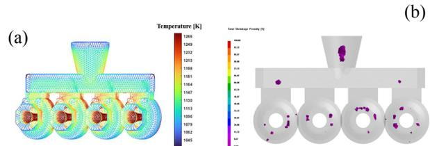
Figure 4 (a) The snapshot of the temperature field of the mold shell with dynamic corrections, (b) Simulation results of the shrinkage porosity in the casting.
