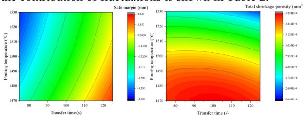
Figure 3 Response surface of safe margin and shrinkage porosity
