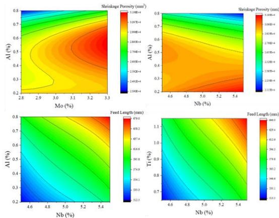
Figure 2 Response surface of shrinkage porosity and feed length.
