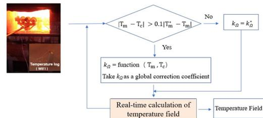
Figure 1 Schematic diagram of dynamic corrections of shell temperature.
