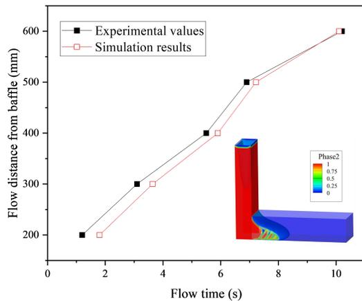
**Figure 2 Comparison between UHPC L-shaped box test and simulation**
