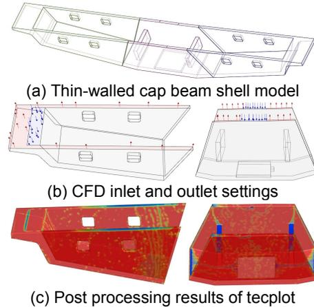
**Figure 3 Thin-walled cap beam shell CFD model and results**
