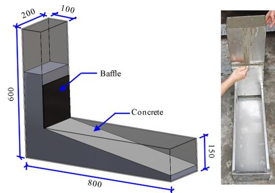
Figure 1 L-shaped box dimensions (unit: mm)
