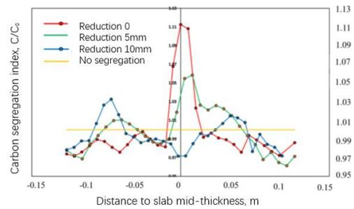
Figure 6 Effect of liquid reduction on macrosegregation
