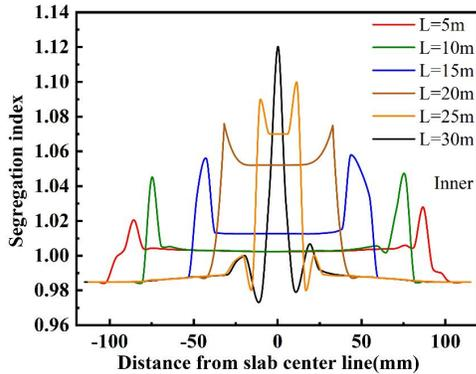
Figure 4 Segregation index at different thickness position to meniscus
