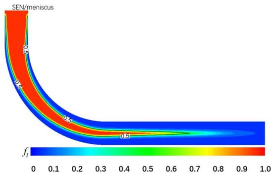
Figure 1 Solidification process of continuous casting slab
