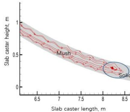
Figure 7 Backflow caused by the mush compression
