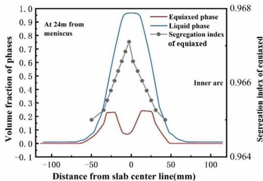
Figure 5 Liquid and equiaxed fractions as well as equiaxed segregation index along thickness
