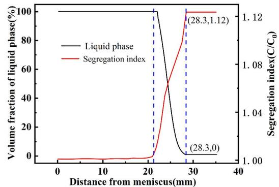
Figure 3 Evolution of liquid fraction and segregation index along casting centerline
