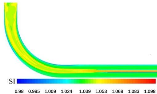
Figure 2 Macrosegregation in continuous slab casting
