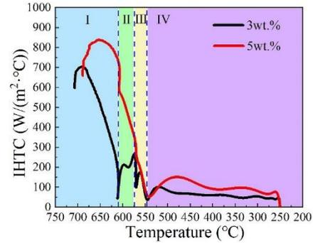
Figure 4 Two types of frozen sand mold IHTC trend with temperature variations
