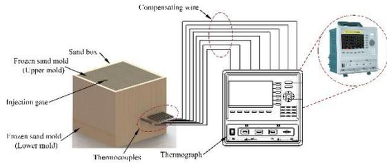
Figure 3 The frozen casting thermometry experiment
