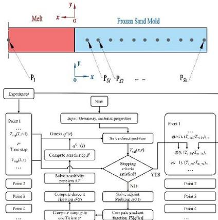
Figure 2 1-D heat transfer assumptions and IHCP inversion modeling calculation procedure
