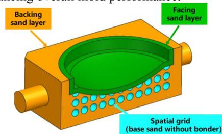
Figure 1 Schematic diagram of cross-section of the spatial meshed sand mold.
