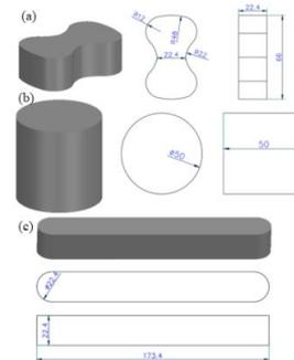
Figure 2 Standard solid sand sample
