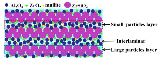
Fig. 3 Formation and strengthening mechanism of printing layer structure.
