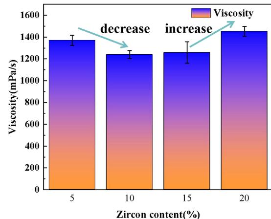
Fig. 1 Viscosity of alumina ceramic slurry with different zircon content: (a)5% (b)10% (c)15% (d) 20%
