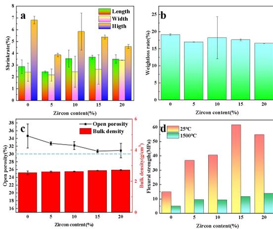
Fig. 2 Properties of alumina ceramic cores with different zircon contents:(a) Shrink rate (b) Weight loss rate (c) Open porosity and bulk density (d) Flexural strength
