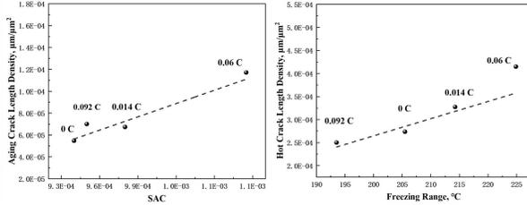
**Figure 1 Relationship between aging crack density and SAC and between hot crack and solidification range.**
