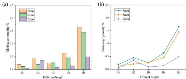
**Fig. 3 The contents of microporosities with different thicknesses and heights of the plates.**
