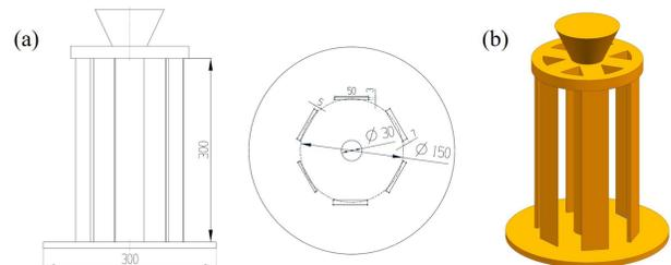
Fig. 1 Schematic diagram of GH3230 thin-wall plates: (a) schematic diagram of size; (b) schematic diagram of three-dimensional model.
