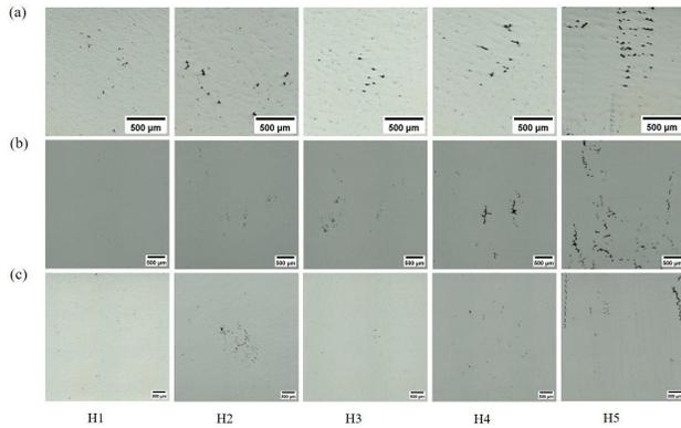
**Fig. 2 Schematic diagram of the plate microporosities with different thickness and height: (a) 3mm plate, (b) 5mm plate, (c) 7mm plate; H1: lower, H2: lower-middle, H3: middle, H4: upper-middle, H5: upper.**
