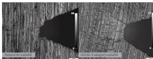
Figure 3 Thermal fatigue tests showed maximum crack length of 120 μm with Fastcool 55 material; and crack length of 500μm with NADCA C category materials.
