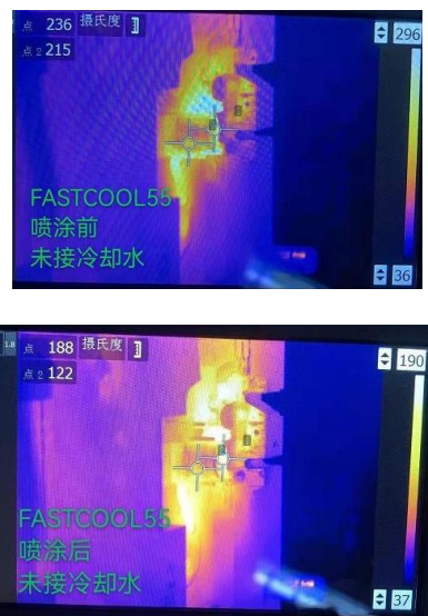
Figure1 Surface temperature of Fastcool 55 material in die casting dies
