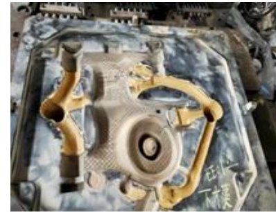
Fig.4 Horizontal pouring channel coated with insulation paint
